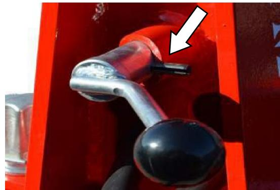
Before begining the transport process, make sure to position the lock pin fixing. (Figure-21).
