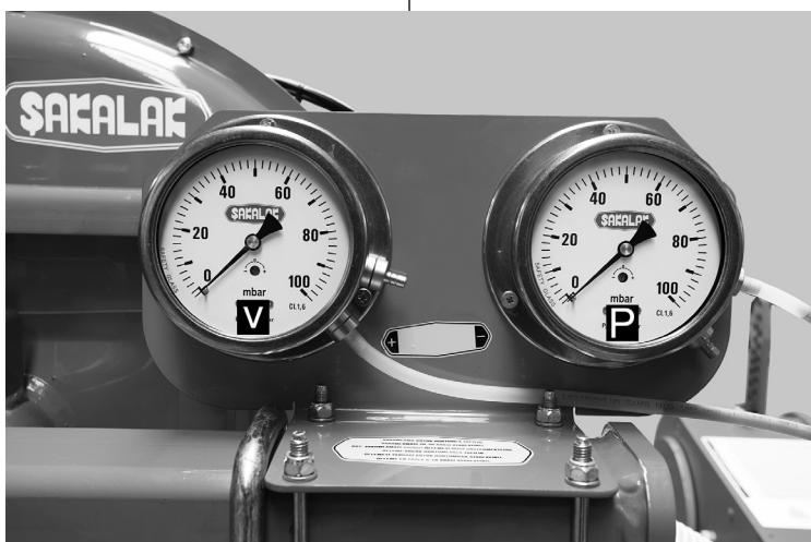
Increase tractor engine speed until required vacuum reading shows on vacuum gauge.
